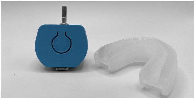
Figure 1. Cwash ® device in its two connecting parts. On the left the mechanical and electrical part, on the right the medical grade polymeric Bite.
